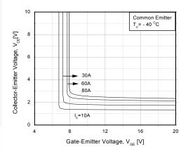
Figure 6. Saturation Voltage vs. V<sub>GE</sub>
