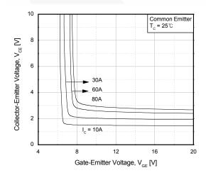
Figure 2. Typical Saturation Voltage Characteristics
